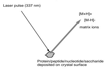
• Sample mixed with a UV-absorbing matrix and is allowed to co-crystallize on the metal target.
