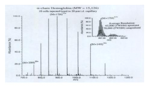
Mass spectrum of hemoglobin obtained by introducing 10 red blood cells into the capillary of a CE-MS instrument.
