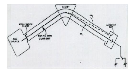
Generated ions are accelerated and are passed around a curved track (the sector) leading to a detector. By increasing the magnetic field applied to the ions, heavier ions with higher momentum can be induced to follow the curved track. A mass spectrum is obtained by applying a magnetic field gradient. Scanning is somewhat slower than in a quadrupole analyzer due to "magnetic reluctance".
