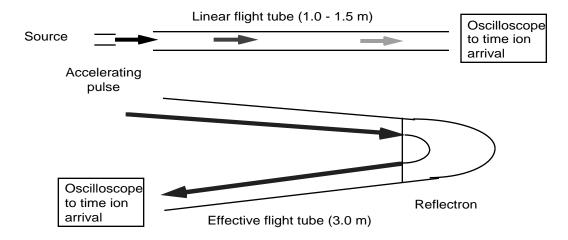
• Generated ions are accelerated so that they have equal kinetic energy. They are allowed to "drift" down a 1 - 1.5 meter tube before striking a photomultiplier detector. The "time of flight" (t) depends on the mass of the ion (m), where
