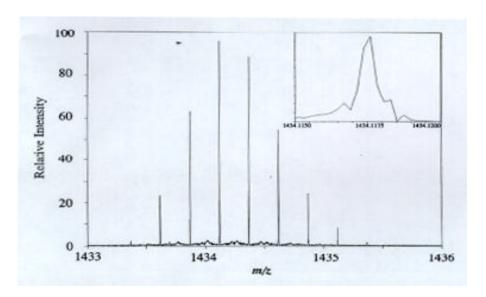
Mass spectrum of bovine insulin showing the separation of the naturally occurring isotopic forms. The mass resolution of the peak shown in the inset is  $> 2.5 \times 10^6$ . Data were collected for 80 sec for this experiment.
