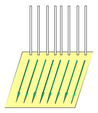
Parallel capture of effluents of 8 nanoLC separations on Mylar - can be scanned simultaneously by fast laser
