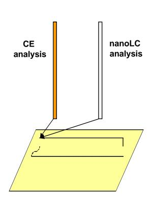
Creates 20 mm wide tracks that can be scanned by MALDI laser for MS analysis
