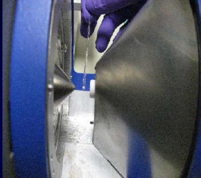
Liquid samples are introduced with a glass capillary tube closed at one end
