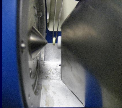
Solid samples are introduced into the stream with tweezers
