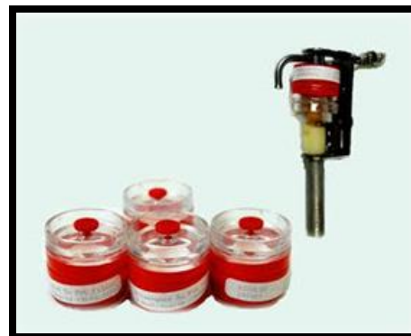
This is an image of a respirable dust sampling (top right) and pre-weighed cassettes for gravimetric sampling (bottom).
