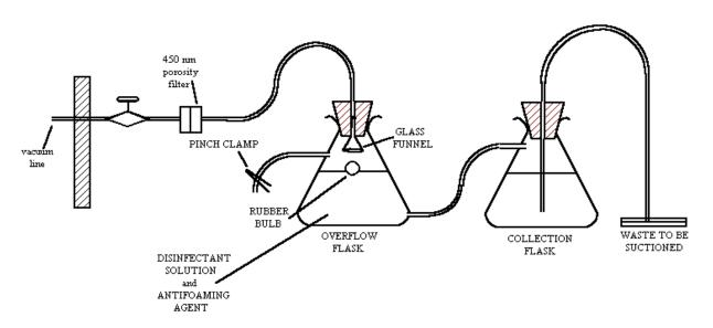
TWO TECHNIQUES FOR PROTECTING VACUUM SYSTEM FROM CONTAMINATION
