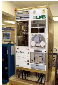
Figure 1: X-ray Crystallography Facility. Includes: X-ray data collection with CCD detector, crystal manipulation/mounting, -180°C freezer & cryo-preservation.
