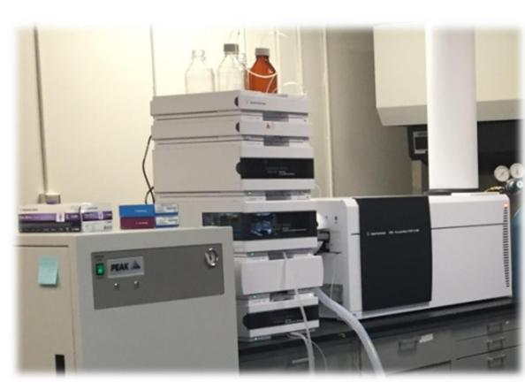
Agilent Q-TOF HPLC-MS: an ultra-high pressure HPLC system with a binary pump, autosampler, two column modules, and a diode array detector. The mass spectrometer is capable of being operated in either MS mode, or MS-MS mode. Compounds can be run by Electrospray or APCI, in both positive and negative ion mode, with a mass measurement accuracy within 2 ppm. This unit is located in Samuel C. Armstrong Hall, Room 101 and managed by Marilyn Tourne, PhD.
